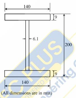
The plastic section modulus about the weaker axis (in cm³, up to one decimal place) is
